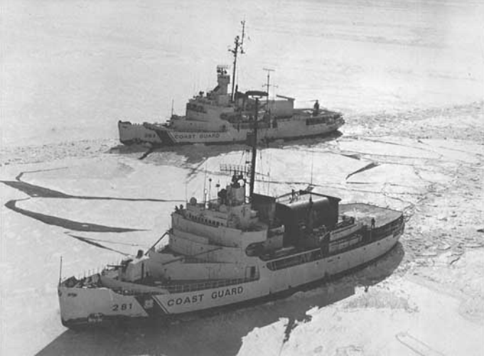
Parallel operation makes icebreaking much faster.
