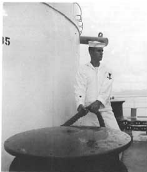
Conklin uses capstan for taking slack out of mooring line.
