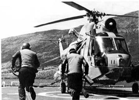
A windy day calls for choks and tie downs as helos come aboard.
